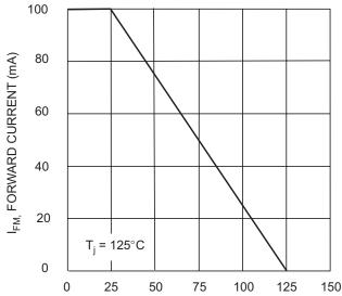
T<sub>A</sub>, AMBIENT TEMPERATURE (°C) Fig. 1 Forward Current Derating Curve
